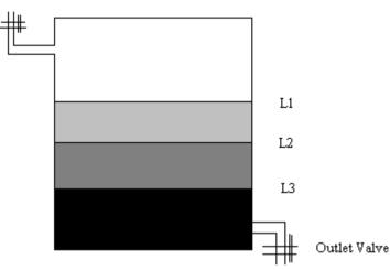
The inlet valve draws water from the main-tank system and the outlet valve sends the surplus water back to the main tank. The water in the main tank must be maintained at a constant value, if the level drops the motor must be turned on.
