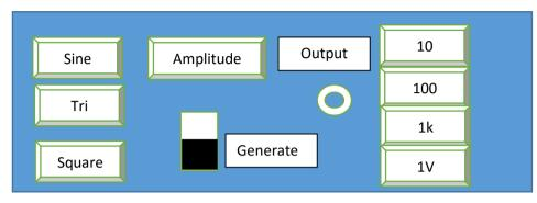
On system power up the user has to configure the desired type of waveform (square/triangle/square), frequency and amplitude.
